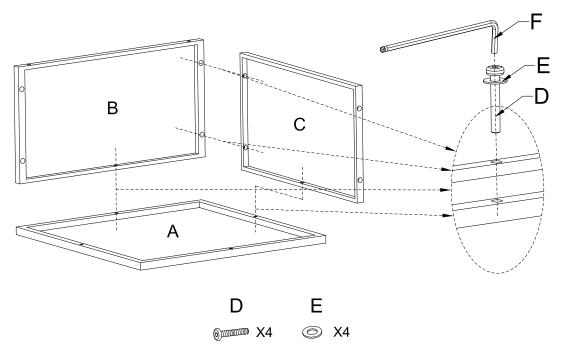
Step 2. Repeat Step 1 to attach 1 pc of Side Panel(B) to Top (A),1pc of End Panel (C) to Side Panel (B) & Top (A)
